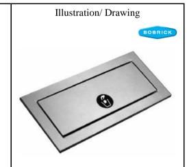
Rough Countertop Cutout 11-1/4" (285mm) wide 4-1/2" (115mm) high 3/4" to 1-1/2" (19 to 38mm) mounting thickness 4-1/2" (115mm) minimum clearance below mounting surface
